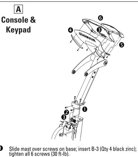
Connect heart rate cable in mast to base and console.
